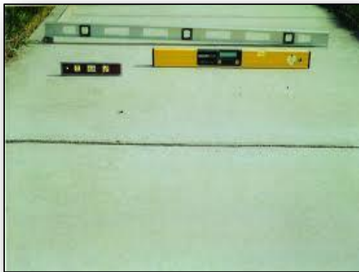
Smart Tool used to measure Cross-Slope
