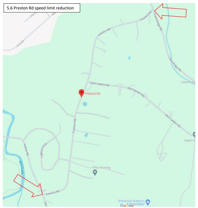
Analysis: Preston Rd is designated as a T3-R-CA3 in Metro's major and collector street plan and has two 10-ft +/- lanes with multiple vertical and horizontal curves. Metro's traffic schedule 2 shows the speed limit for Preston Rd as 40 mph from Pettus Rd to Cane Ridge Rd.
