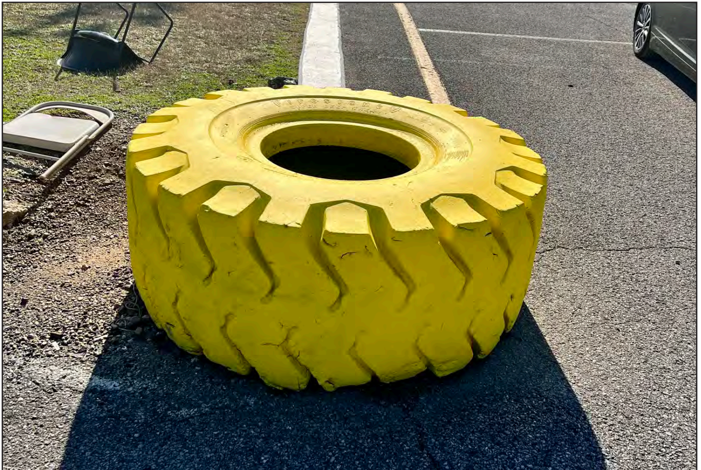
Heavy machinery tyres currently used as attenuator
