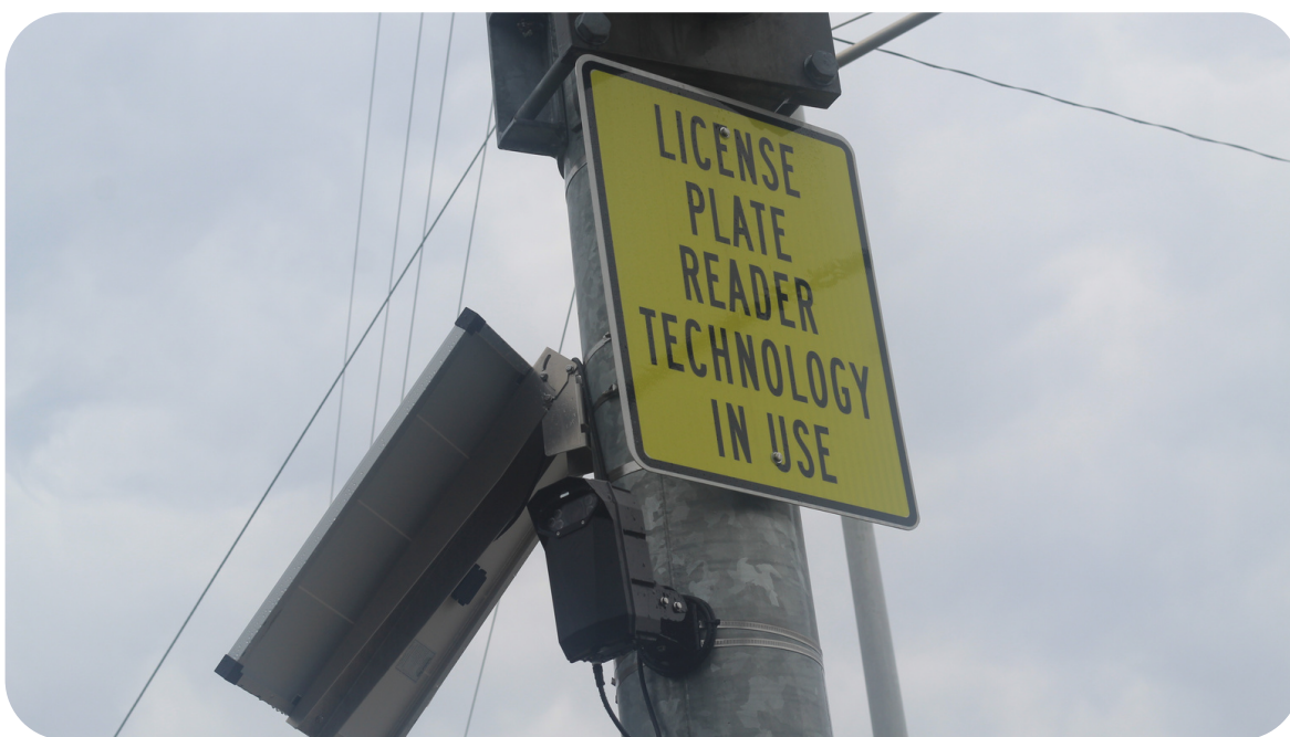
Photo 1: A LPR camera and its signage in use in Nashville, captured by MNCO staff.
