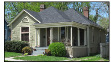
In many districts, windows are generally twice as tall as they are wide.
