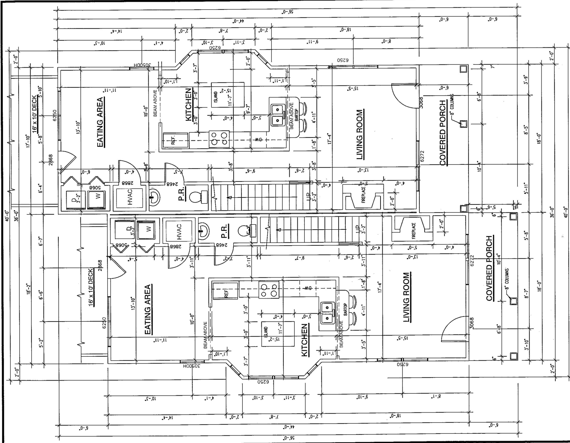
**FIRST FLOOR PLAN** 9'-0" FIRST FLOOR CEILING HEIGHT
