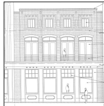
Figure 2: Proposed 2<sup>nd</sup> floor windows are similar to the MDHA design previously approved and seen above.
