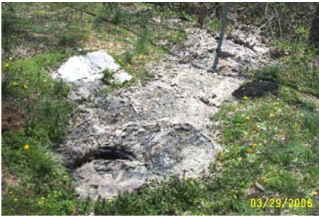
Sanitary Sewer Overflows caused by fats, oils and grease.
