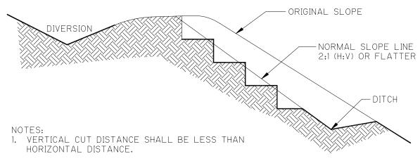
2. VERTICAL CUT SHALL NOT EXCEED 24" (600 mm) IN SOFT MATERIAL AND 3' (1 m) IN ROCKY MATERIAL.
