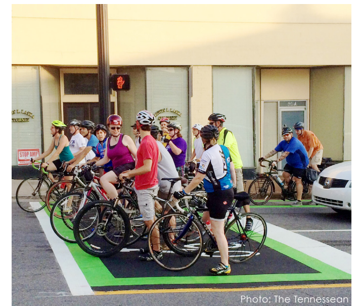
Church Street (installed 2014): Bike box
