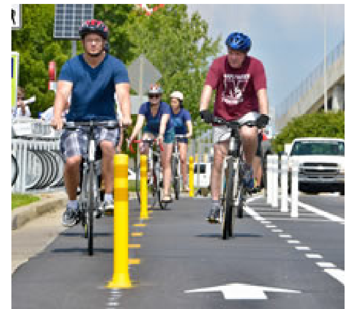
Davidson Street (completed 2015): 1.8 mile at-grade cycle track
