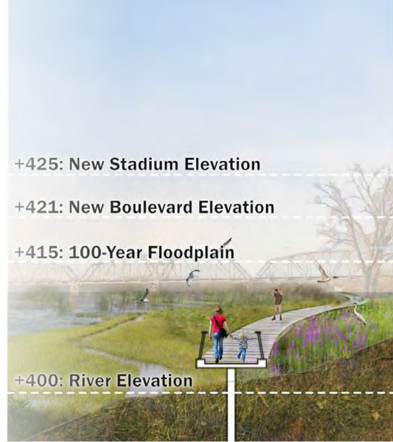
Underlying the design for Central Waterfront Park is a riparian framework that slows and stores stormwater and lays back the river’s edge to reduce flooding.
