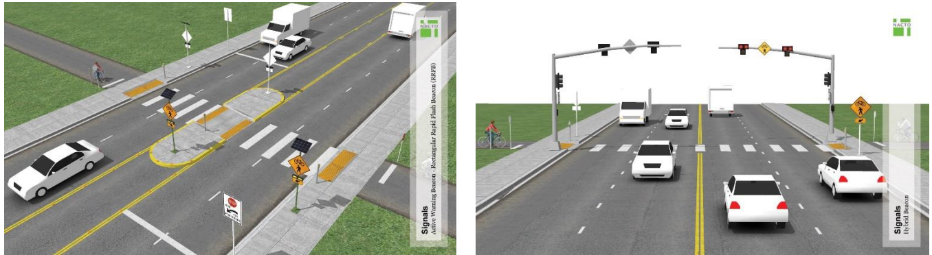
Figure 41. Rapid Rectangular Flashing Beacons (RRFB) and High Intensity Activated Crosswalks (HAWK)
