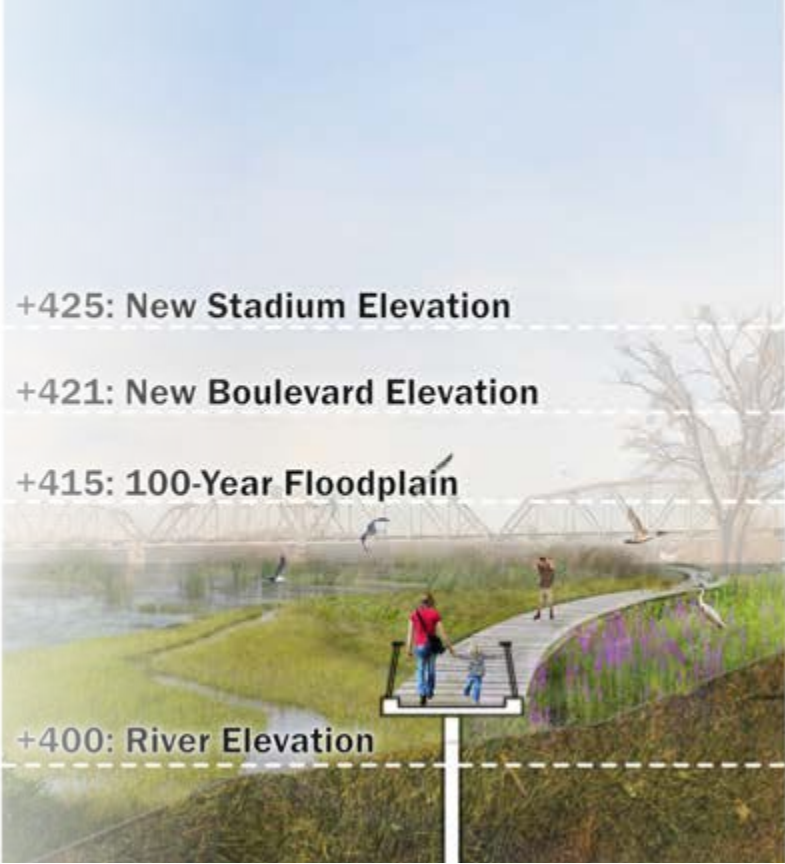
Underlying the design for East Bank Park is a riparian framework that slows and stores stormwater and lays back the river’s edge to reduce flooding.
