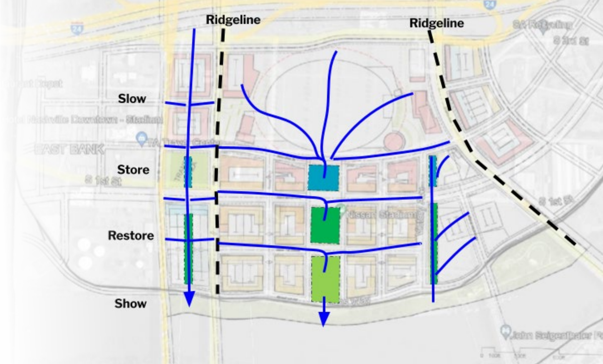
Early concept sketch of utilizing outdoor park spaces within a district stormwater system on the East Bank.
