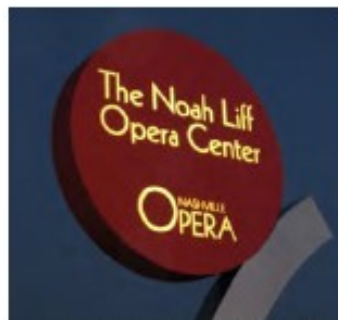
Internally lit cabinet signs with darker background
