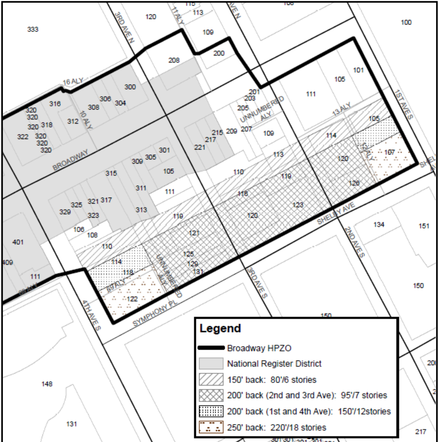
Map showing general areas of additional height. (Measurements should be taken from the front property line along Broadway.)
