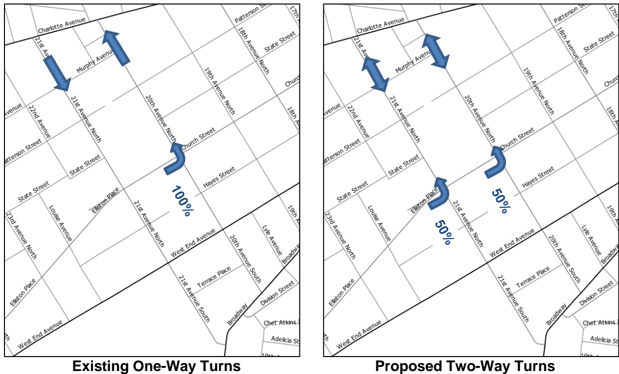
FIGURE 23: EXAMPLE LEFT TURN DISTRIBUTION
