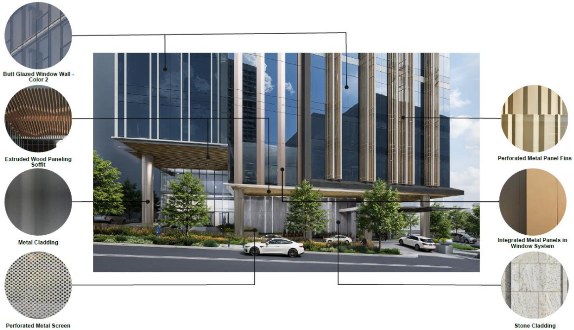
Figure 10: Northern façade material callouts
