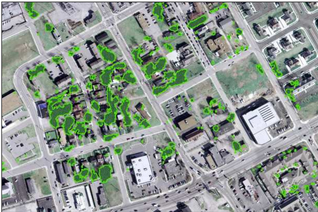
Figure 3.24--Tree Canopy Cover Polygons Mapped From 1-Meter NAIP Imagery.
