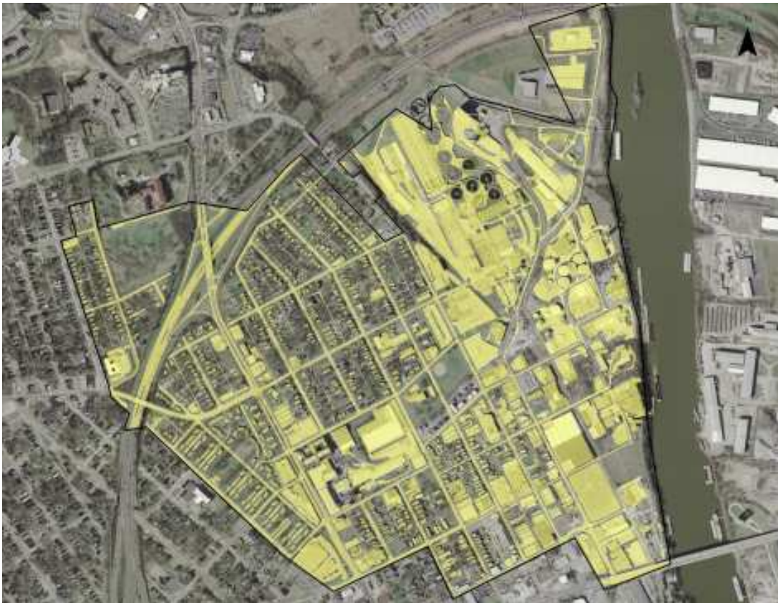
Figure 3.45—Impervious Area in the Van Buren CSS Basin.
