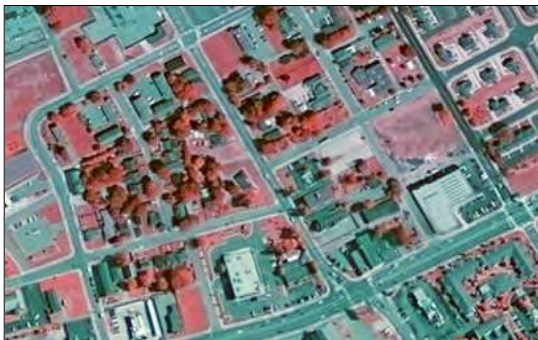
Figure 3.22—One Meter Resolution, NAIP Image Viewed In False Color (Color-Infrared).
