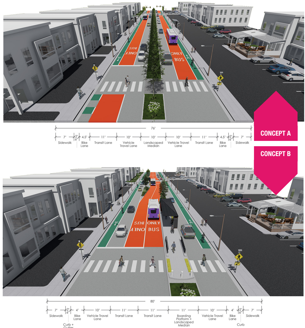
Figure 13. Typical Sections for Main Street from South 5th Street to Eastland Avenue
